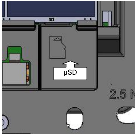
Fig. 8 cVEND box - microSD memory card insertion
